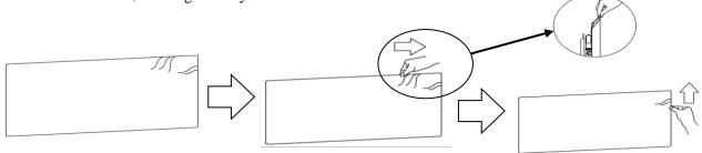
**Incorrect material installation** –The corners of the screen material are not properly wrapped along the edge of the frame leaving the material with unbalanced tension and an uneven finish. To correct, detach springs from material at the corner(s) where material does not lie flat along the edge of the frame, reposition the material so that it lies flat and wraps along the edge of the frame, and reattach springs to the material.
